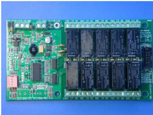
VIO-485: Relay Controller Board
